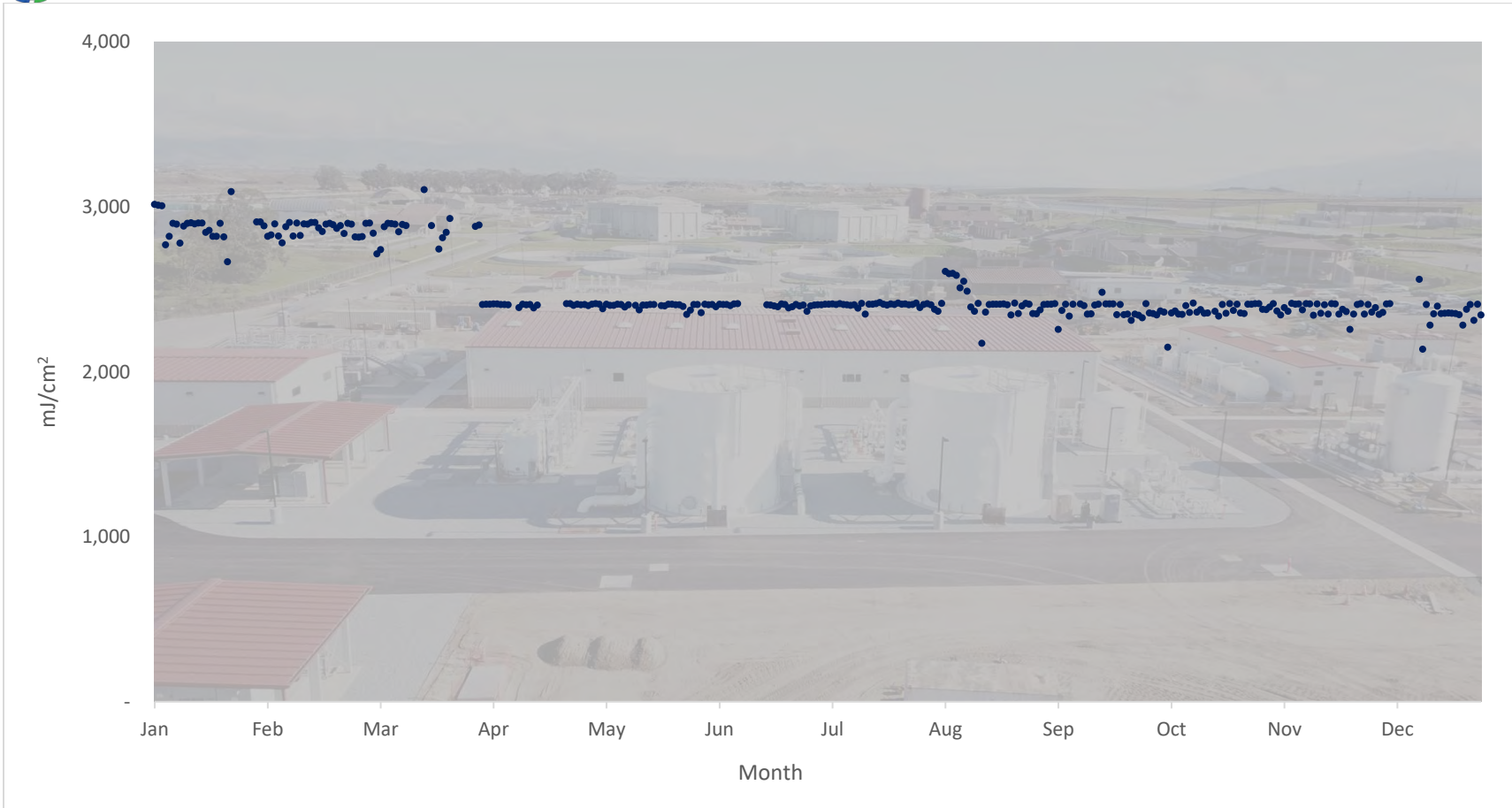
Figure 42. AWP Product Water Monitoring – Daily Minimum UV Dose for Reactor 3 (mJ/cm 2 )
